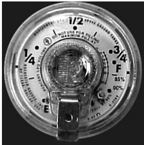
LP Tank Gauge
