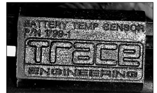
Battery Temperature Sensor.
